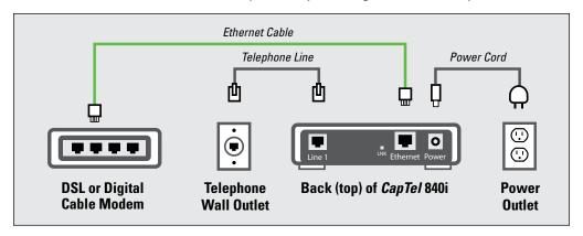
**Example 2:** If there is not an available Ethernet jack in your DSL or Cable Modem, you will need a router or switch that lets you connect more than one device to the Internet. Contact your Internet Service Provider for information about what router or switch will work with your modem. The router should support DHCP. Connect the router to your DSL/Cable Modem. Then connect the *CapTel* 840i to the router or switch using the Ethernet cable as shown below.
