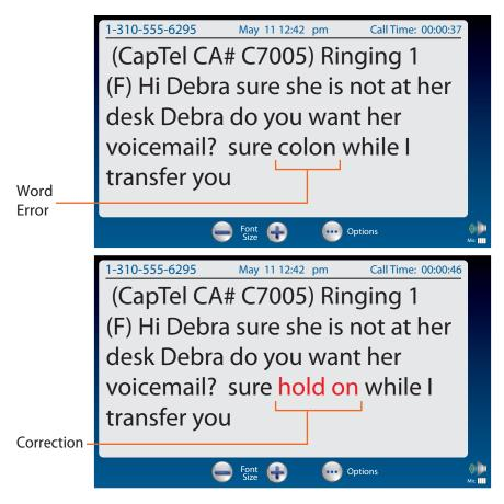
On occasion, word errors may appear in the captions due to the speech recognition system the Captioning Service uses. The Captioning Service will try to correct word errors as they occur. The corrected word appears in a different color than the rest of the captions to let you know a correction has been made.
