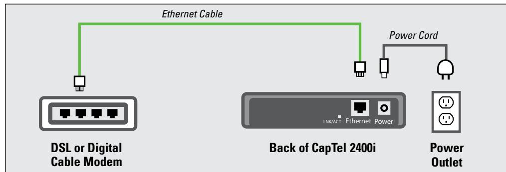
**Example 2:** If there is not an available Ethernet jack in your DSL or cable modem, you will need a router or switch that lets you connect more than one device to the Internet. Contact your Internet Service Provider to learn what router or switch will work with your modem. The router should support DHCP. Connect the router to your DSL/cable modem. Then connect the CapTel 2400i to the router or switch using the Ethernet cable.
