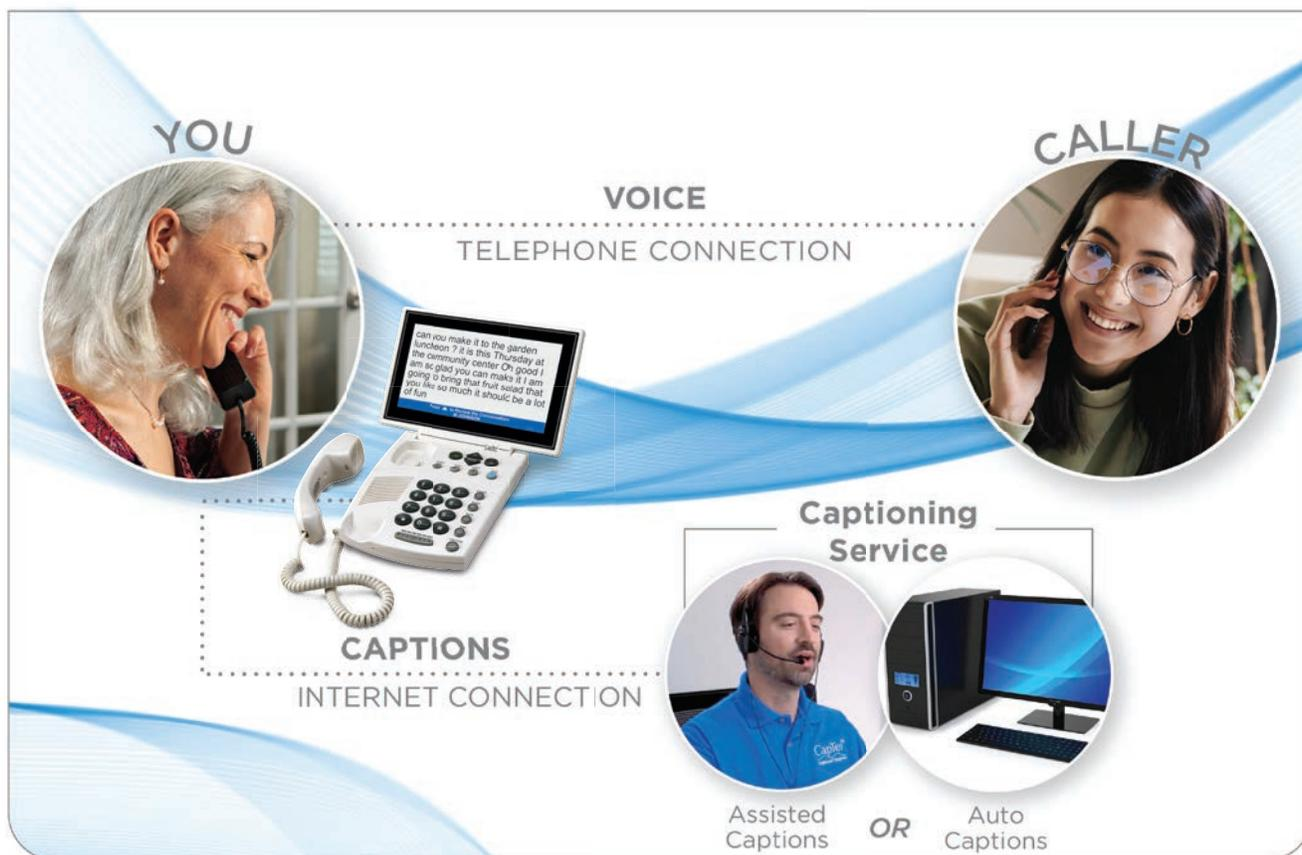
The *CapTel* 880i connects to both your telephone service and to your Internet service. Every time you make a telephone call, the phone uses the Internet connection to access a no-cost Captioning Service. The Captioning Service uses speech recognition technology (either automated or operator-assisted) to create captions of everything your caller says. The captions appear on your *CapTel* 880i display screen for you to read.
