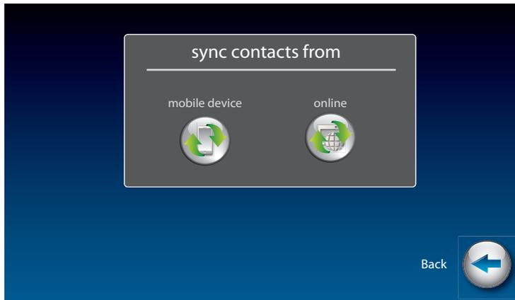
You can transfer contacts from your mobile phone, such as an iPhone or Android device, into your CapTel 2400iBT. CapTel connects to your mobile device via Bluetooth to import the contacts, including pictures. You can select up to 100 contacts from your mobile device to store in your CapTel phone. Each contact entry can have a mobile, business, and home phone number associated with it.
