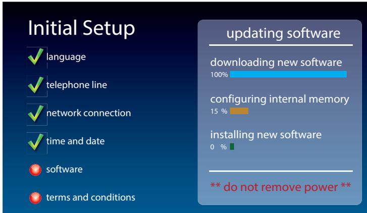
**NOTE** *Do not interrupt the power supply during a software download. It may damage your CapTel phone.*
