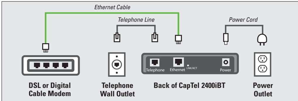
**Example 2:** If there is not an available Ethernet jack in your DSL or cable modem, you will need a router or switch that lets you connect more than one device to the Internet. Contact your Internet Service Provider to learn what router or switch will work with your modem. The router should support DHCP. Connect the router to your DSL/cable modem. Then connect the CapTel 2400iBT to the router or switch using the Ethernet cable.
