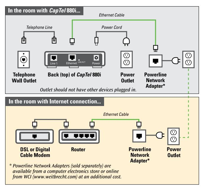
**IMPORTANT:** The Powerline Network Adapters cannot be plugged into a power strip, surge protector, extension cord or GFI-type outlet. They must be connected directly into the electrical wall outlet.
