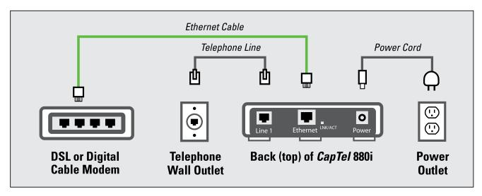
**Example 2:** If there is not an available Ethernet jack in your DSL or Cable Modem, you will need a router or switch that lets you connect more than one device to the Internet. Contact your Internet Service Provider for information about what router or switch will work with your modem. The router should support DHCP. Connect the router to your DSL/Cable Modem. Then connect the *CapTel* 880i to the router or switch using the Ethernet cable as shown below.
